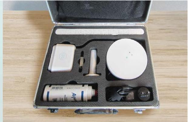
All equipment needed in the OsCare Sono® measurement are conveniently carried in the case: the measurement device, measurement aids (ruler, patient's hand support and ultrasound gel) as well as a laptop and its power cord.
