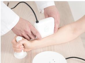
The OsCare Sono® is a novel, low frequency ultrasound device for screening of osteoporosis. The device assesses an individual's bone strength by measuring the axial transmission speed of ultrasound in the forearm radial bone. OsCare Sono® offers a simple, inexpensive solution for screening of osteoporosis without exposure to X-rays.
